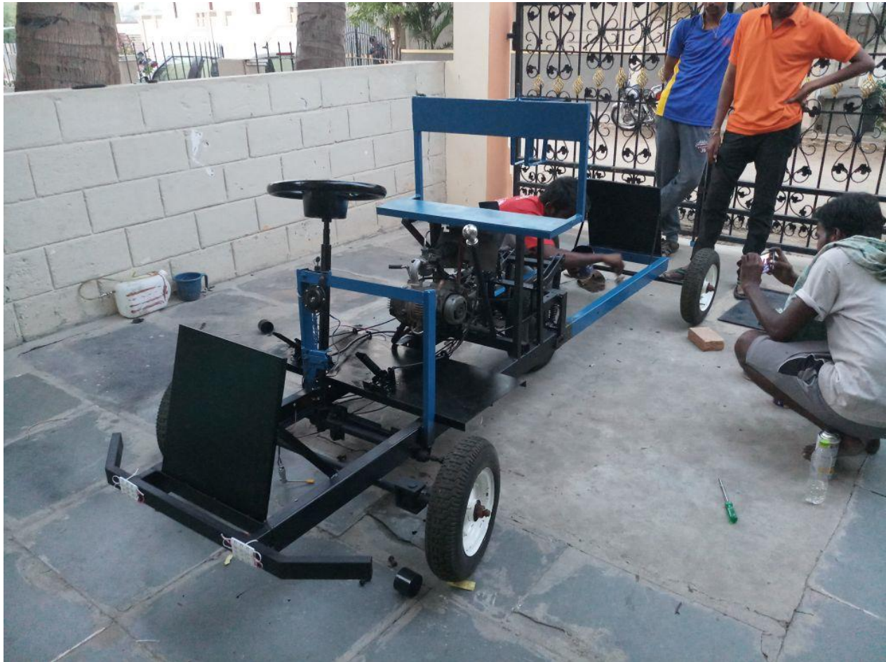
Design and Fabrication of Five Wheeled, Single Wheel Driven, Extension Chassis Transit Vehicle
