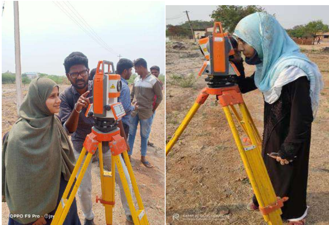
Plate 1 & 2:- Staking out points by using total station
