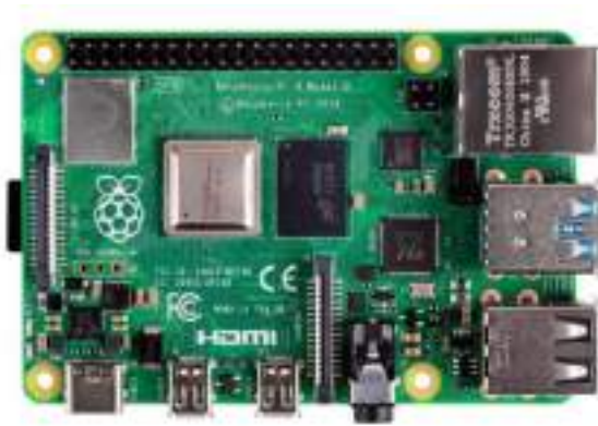
Fig-2: Circuit of Raspberry Pi-4 Model B
