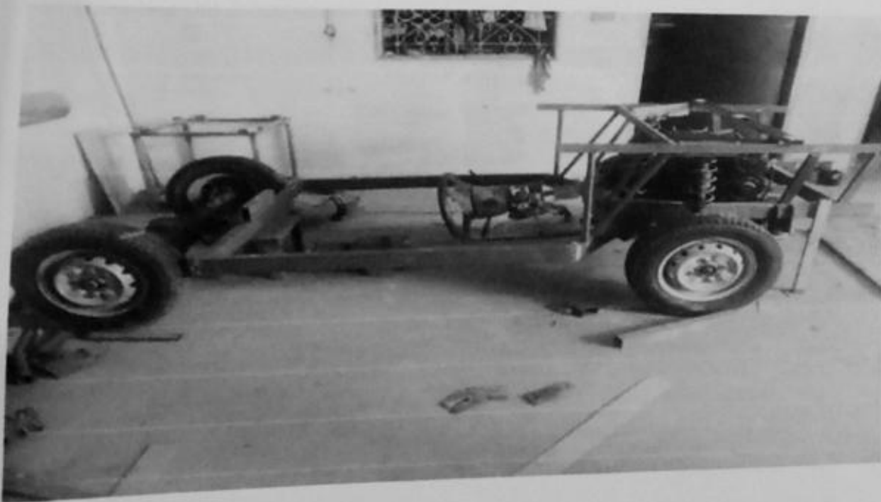
Figure 7.4- Assembling of front and rear wheel drives on chassis.
